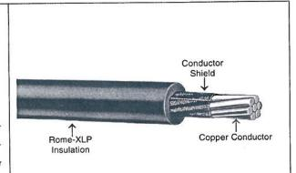
CONSTRUCTION: Annealed uncoated copper conductor, conductor shield, Rome-XLP black thermosetting chemically crosslinked polyethylene insulation, surface printed.
